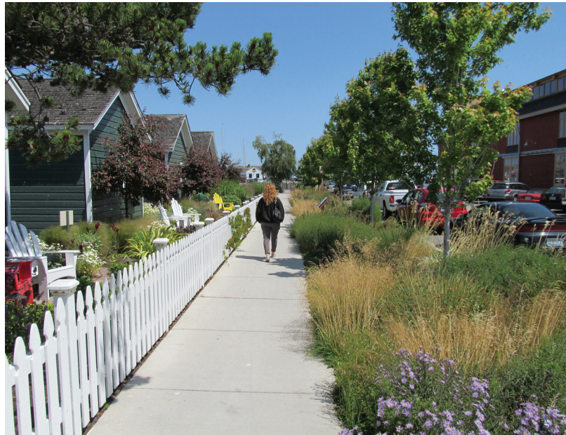
above: bioswale and sidewalk
